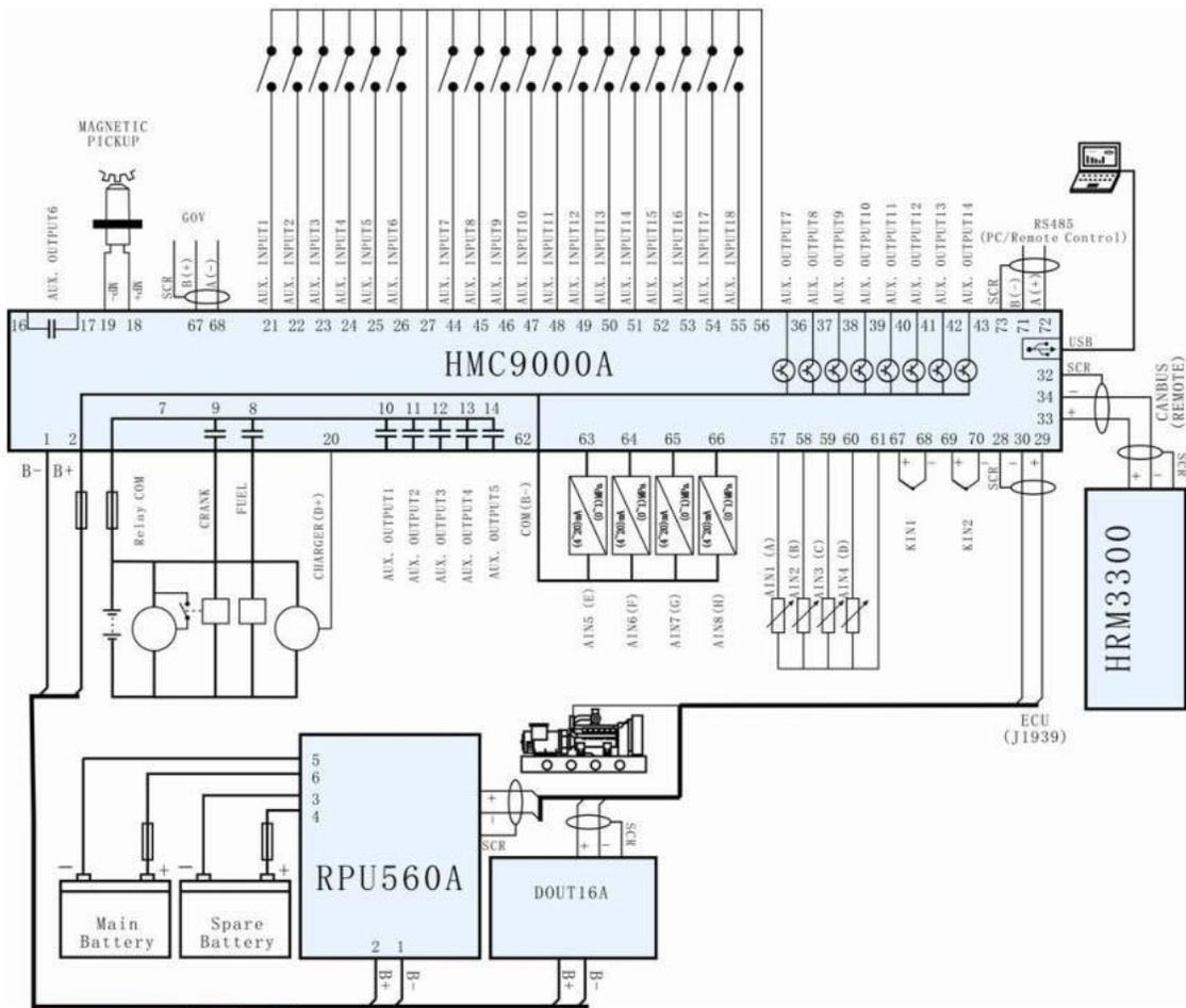
**HMC9000A Typical Wiring Diagram**
