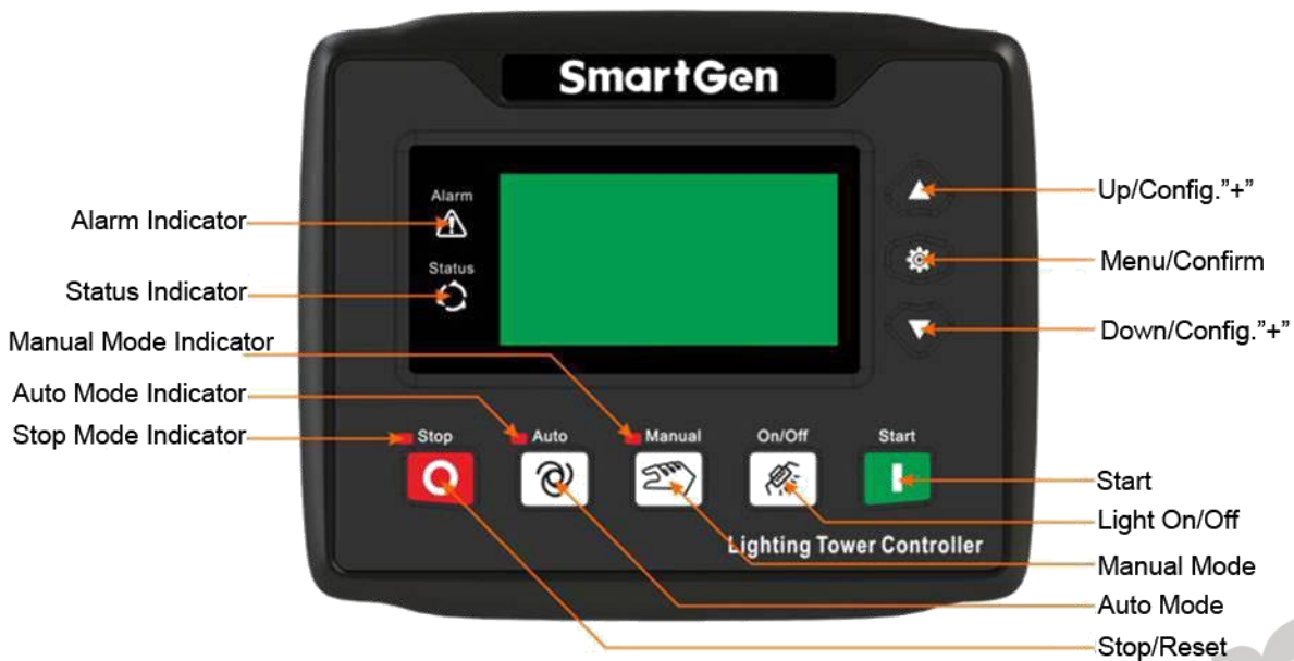
Fig.1 - ALC404 Front Panel
