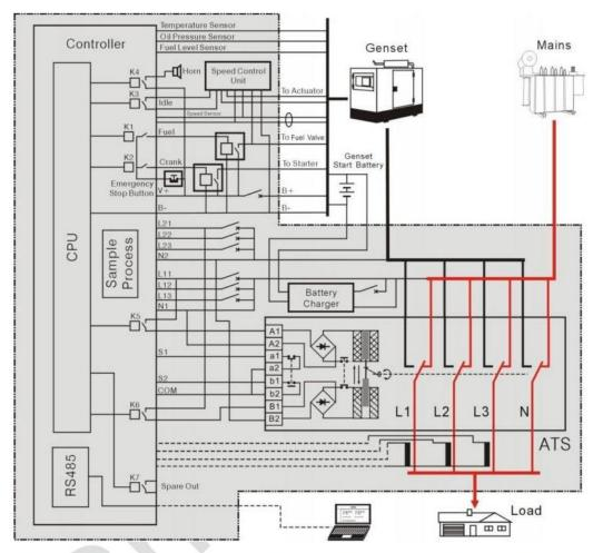
Note: The above drawing is suitable for N type and T type switch (SGQ), please refer to SGQ instruction for more details about M type switch.
